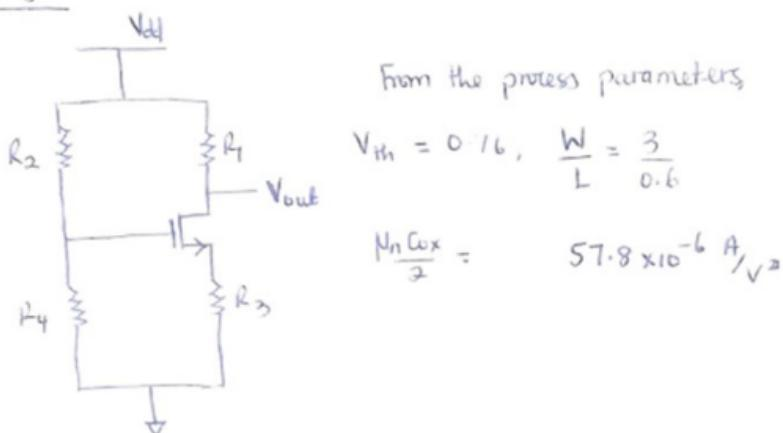
$$\rightarrow V_G = V_{dd} * \frac{90k}{(90+10)k} = \frac{90}{100} \times 10 = 9 \text{ V}$$
