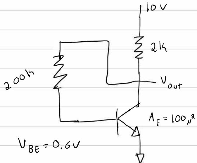
$$i_b = \frac{V_{out} - 0.6}{200k}, \quad i_c = \beta_n i_b$$
